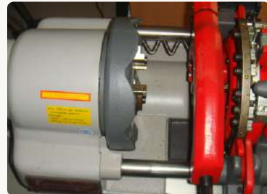
Rothenburger Tap Threading machine used for high speed, High capacity tap threading onto Schedule 40 & Galvanised iron Pipes, Mobile & rugged suitable for Pipes from 15mm-50mm.
