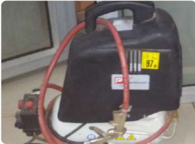
Air Compressor used for air powered tools & calibration of air Vessels on the jorkey Pump of a Three-way fire Pump set.
