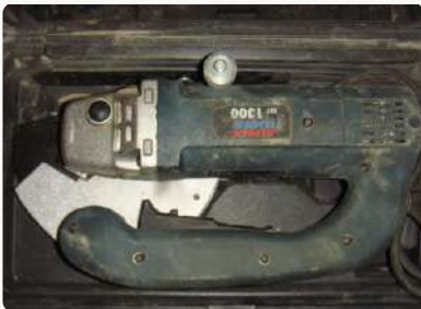
Block work grooving machine capable of adjusting depth of groove to prevent hitting subsurface components e.g. Conduits, anchors Cable etc.
