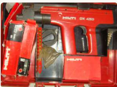
HILTI Ballistic Nail Gun, used to fasten anchors into deep set reinforced Concrete soffits, beams, columns or ambarkments.
