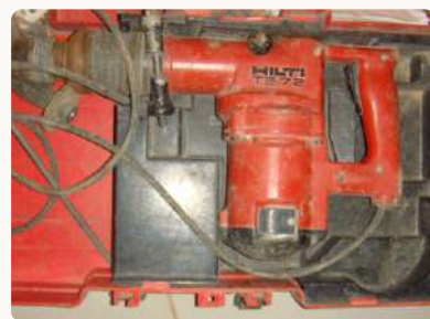
HILTI Te72, High Powered Drill & Hammer
