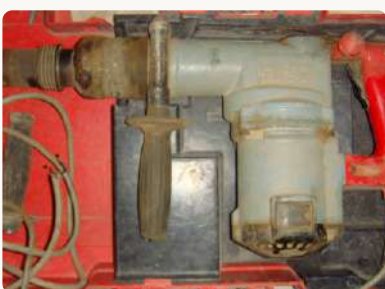
HILTI Te72, High Powered Rotary Drill & Hammer for Boring, drilling & demolition works on any site
