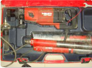
HILTI Diamond Coring rig Capable of Coring through Concrete and Reinforcement with single or double reinforced to a depth of 600mm
