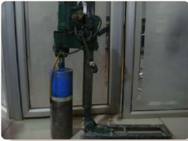
Concrete Coring Machine
