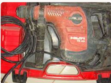
HILTI Rotary Hammer & drill, used for preparation of site for Anchoring fastener and hanging of Pipes & drilling block works.
