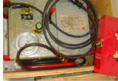
Hydraulics Panel and Console for Control of the Butt Welding Process
